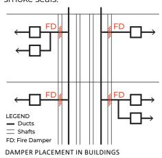
Services like air conditioning, plumbing, and electrical systems often pass through these compartments. Each penetration must be sealed with a compliant passive fire protection system to preserve the integrity of the fire barrier.
