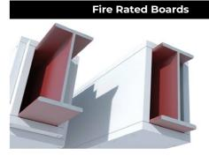
Fire-rated boards can be framed around steel or timber structures in order to fire protect structural members. The composition of boards will differ between manufactures however their general composition is made up of processed gypsum.
