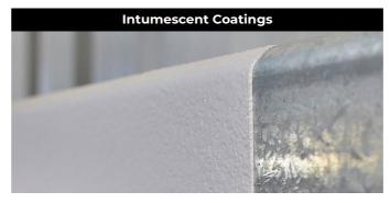
Intumescent is the newest fire protection methodology to come onto the market. Unlike boards and vermiculite, intumescent is a reactive material which expands to insulate structural steel in a fire event. Every intumescent has different material properties and therefore have different required thicknesses and expansion behaviour.
